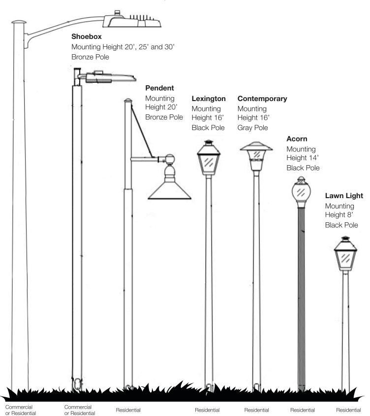
These drawings are not to scale, but are reflective of height differences between different types of fixtures.
