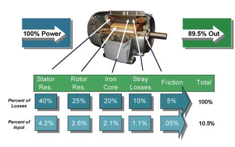
A bad repair/rewind can adversely affect all motor characteristics, reducing efficiency and reliability and producing more damaging heat.
