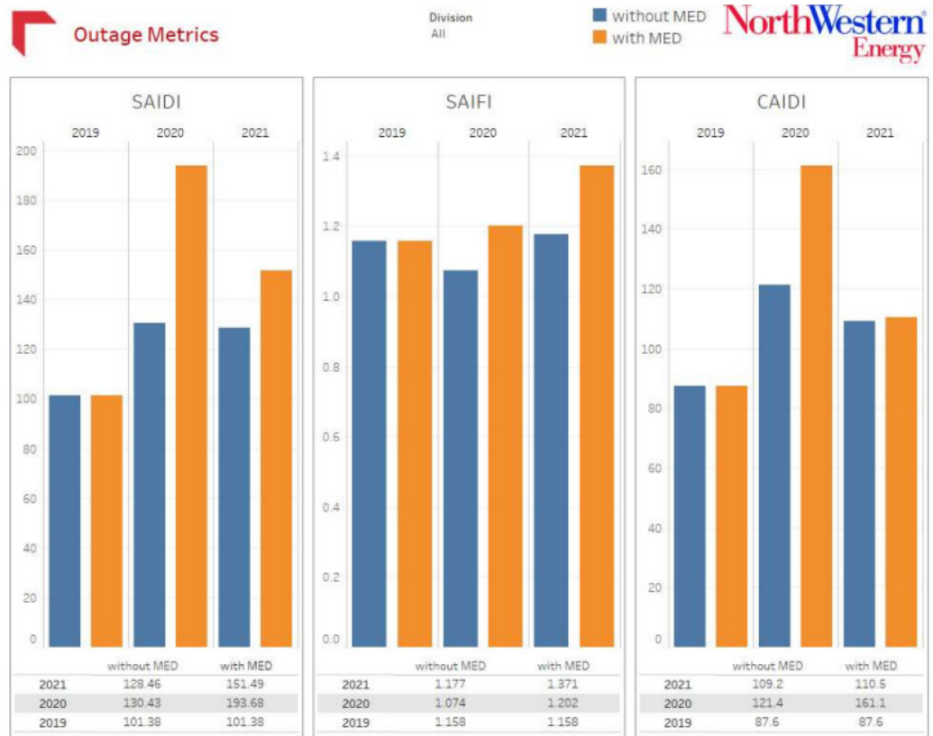
FIGURE 9: MONTANA SYSTEM INDICES WITH AND WITHOUT MAJOR EVENT DAYS (MEDS) AS DEFINED IN IEEE STANDARD 1366-2012.
