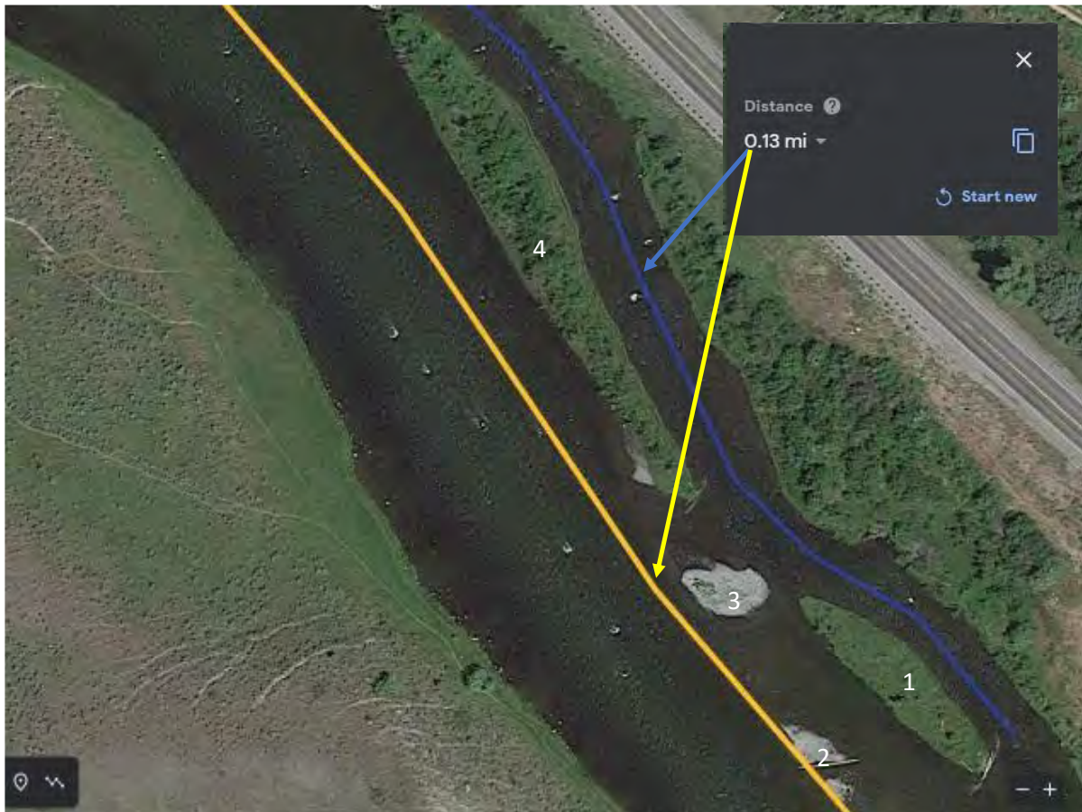
Figure 20. Satellite imagery from Google Earth used to determine channel lengths and covariate densities within sub sections of long-term Madison monitoring reaches. The blue line represents a side channel
