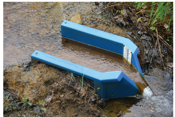
Portable Weir on a Small Stream
