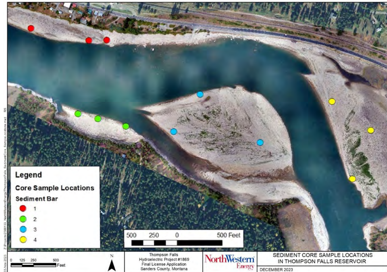
Figure 6-10: Sediment core sample locations in Thompson Falls Reservoir on 7/13/20.
