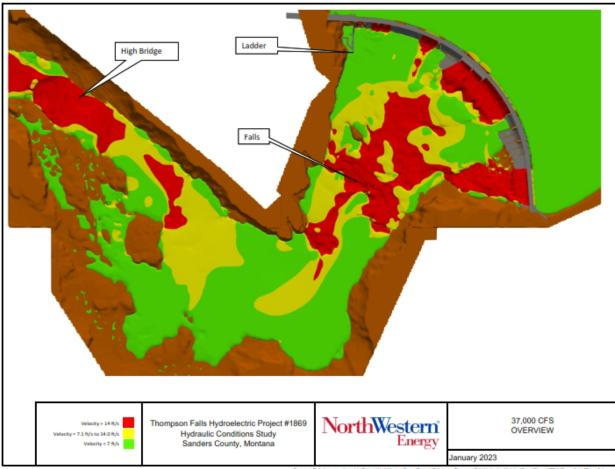
Figure 3-34. CFD Modeled Velocity at 37,000 cfs Spill.
