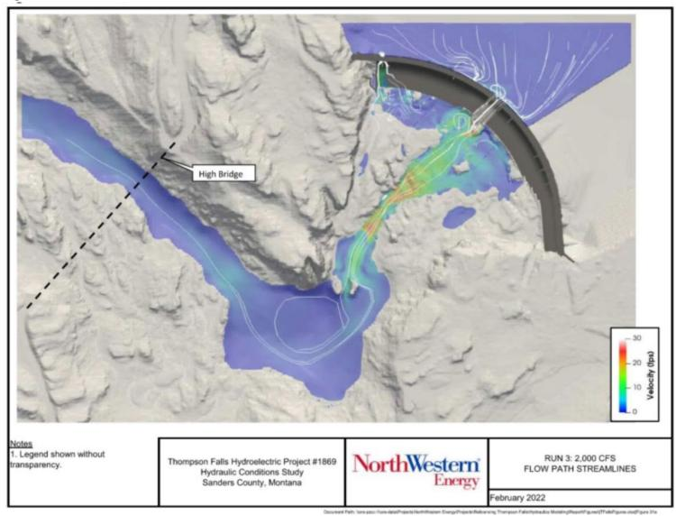
Figure 3-31 Flow Path Streamlines, 2,000 cfs at the Main Dam.
