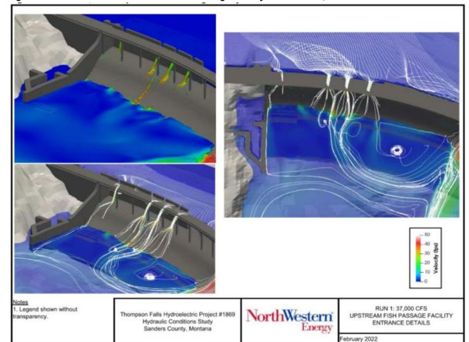
Figure 3-40. Flow Path Details at the Fish Passage Facility Entrance: 37,000 cfs.
