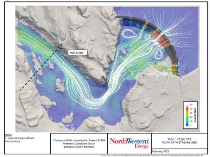
Figure 3-39. Flow Path Streamlines, 37,000 cfs.
