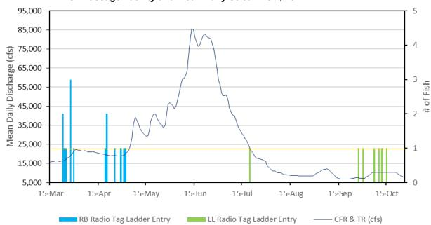
Figure 3-18. Summary of Individual Radio Tagged Rainbow Trout and Brown Trout Entering the Fish Passage Facility and Mean Daily Streamflow, 2022.
