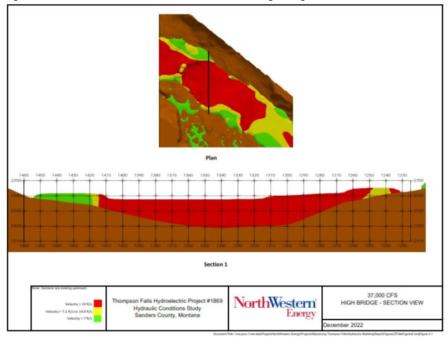
Figure 3-35. Model Scenario, 37,000 cfs. Cross-section at High Bridge.
