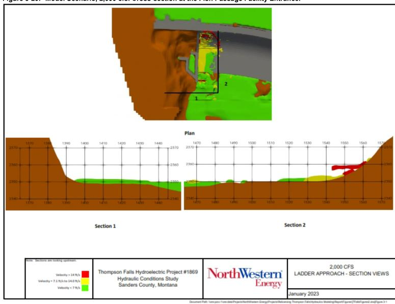
Figure 3-29. Model Scenario, 2,000 cfs. Cross-section at the Fish Passage Facility Entrance.
