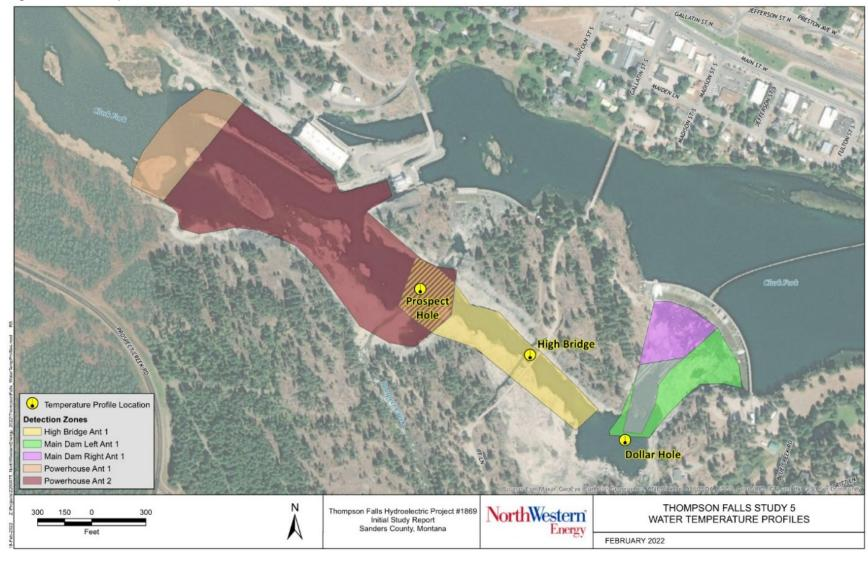
Figure 3-20. Temperature Profile Locations and Fixed Station Detection Zones.
