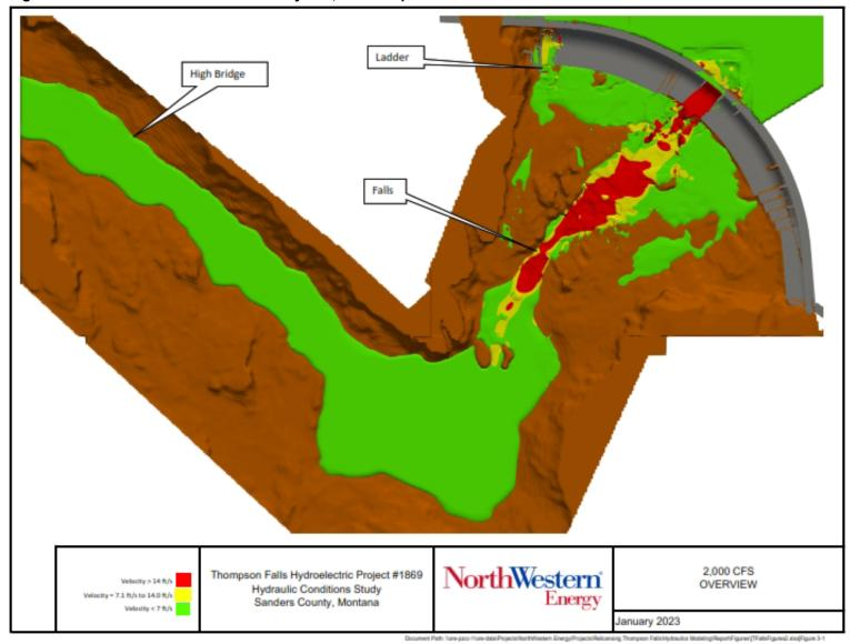
Figure 3-26. CFD Modeled Water Velocity at 2,000 cfs Spill.
