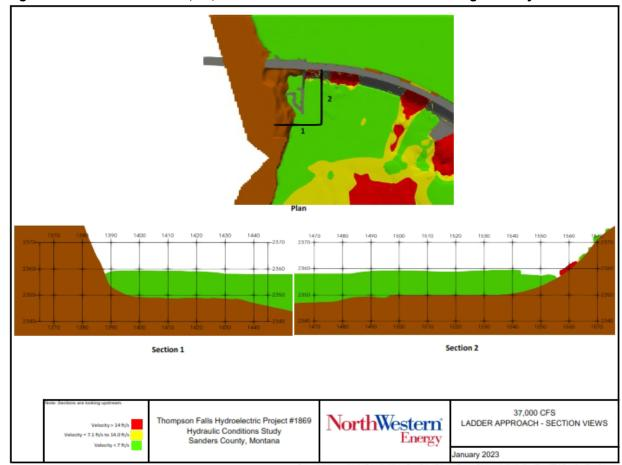
Figure 3-38. Model Scenario, 37,000 cfs. Cross-section at the Fish Passage Facility Entrance.
