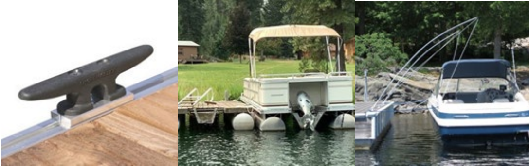
Photo 3-23. Images of Cleat, Boat Tied to cleats, and Boat Secured with Whips
