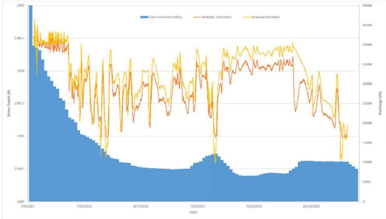
Figure 3-9. Water Surface Elevations at Wetland 1 Compared to Reservoir Elevations and Clark Fork River Inflows.
